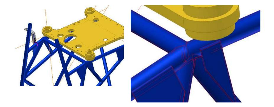
The perfect tube-construction of the engine-mounting.
